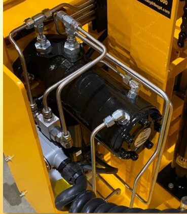
Side rotation anti-drift brake motor
