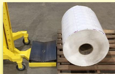
V-Pan shown flush against a standard pallet
