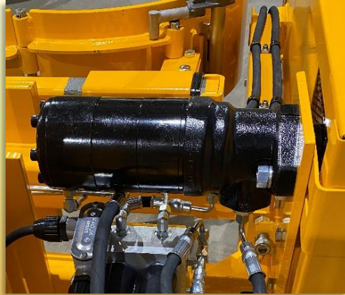
Forward rotation anti-drift brake motor
