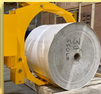
LRCR clamp picking or placing a horizontal roll
