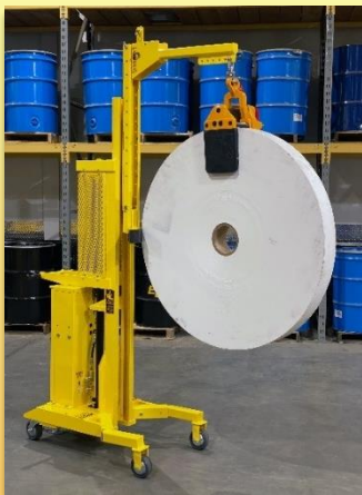
DC Powered Roll-Transporter with Abaco-Style clamp holding roll
