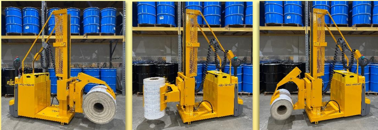
SRCR inner pin position clamping range 12" (30 cm) to 22" (56 cm) in dia.
