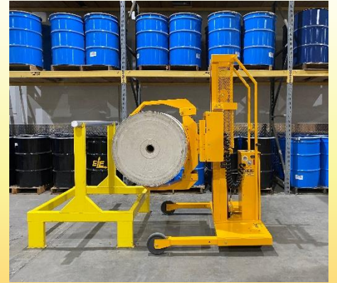
ER straddle leg model with RCR2336-16 clamp with a roll
