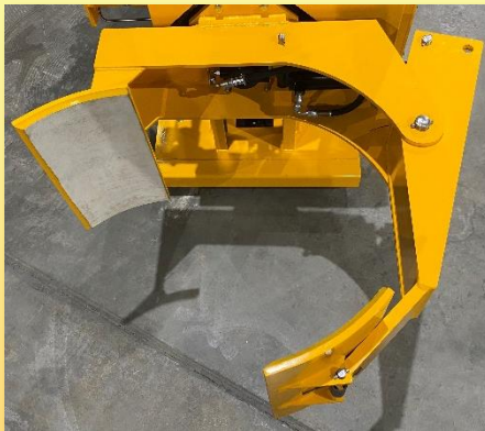
SRCR inner pin position clamping range 12” (30 cm) to 22” (56 cm) in diameter
