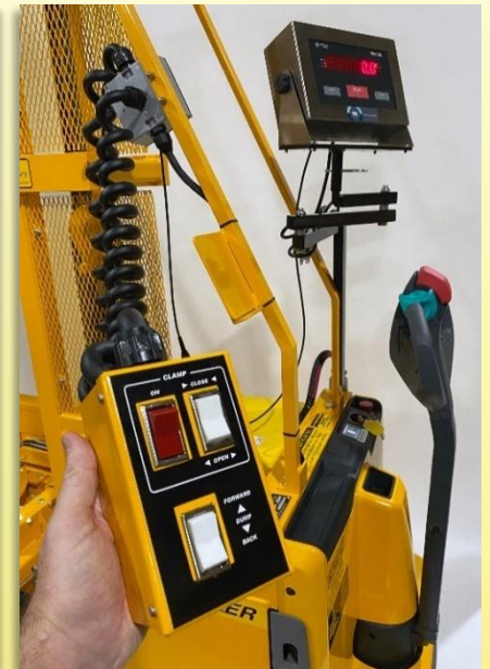
The Remote-Control Box at the end of the coiled cord
