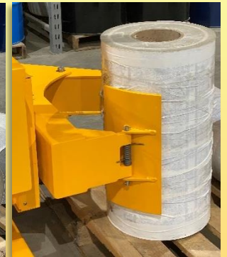
SRCR clamp picking or placing a vertical roll
