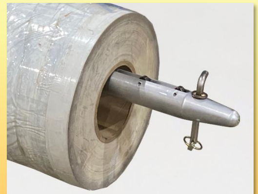
Close-up of Roll Post with Rollers Safety Pin Securing a Roll
