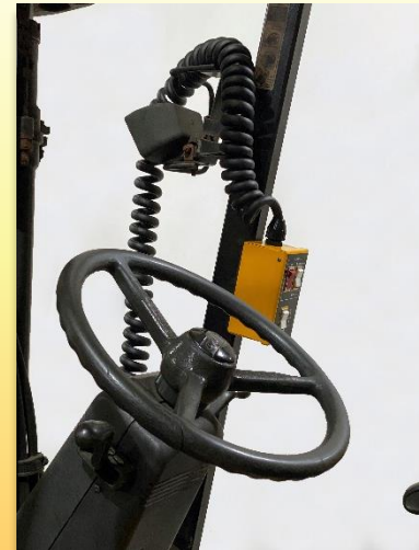
The remote-control box mounted magnetically within a lift truck
