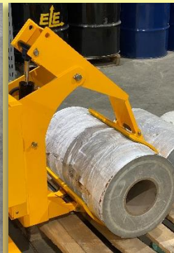
SRCR clamp picking or placing a horizontal roll
