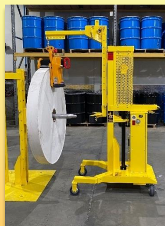
Abaco-style clamp loading roll onto post
