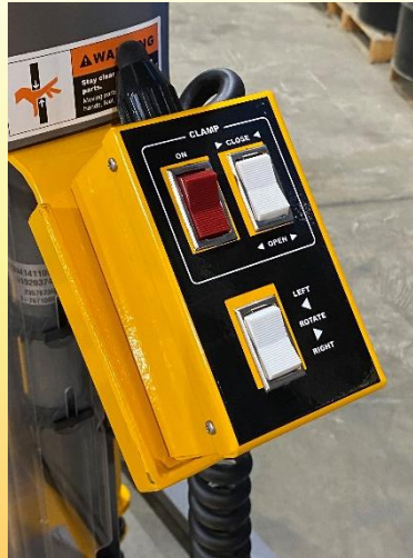
The remote-control box mounted magnetically on a walkie stacker
