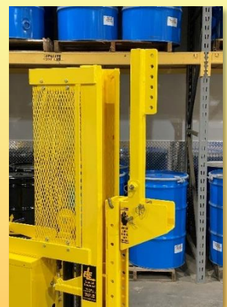
Folding Jib in vertical storage position
