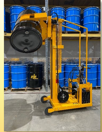
ED Air powered counterbalanced model w/ RCR1324-8 clamp
