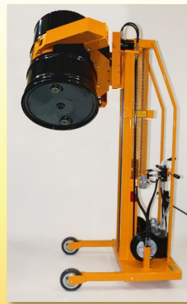
ED Air powered straddle leg model w/ RCR1626-8 clamp
