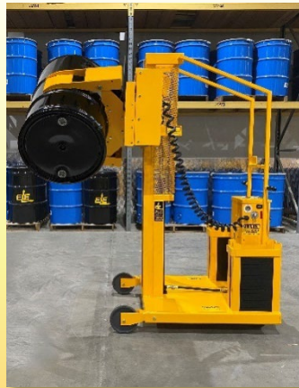
ED DC powered counterbalanced model w/ RCR1324-8 clamp
