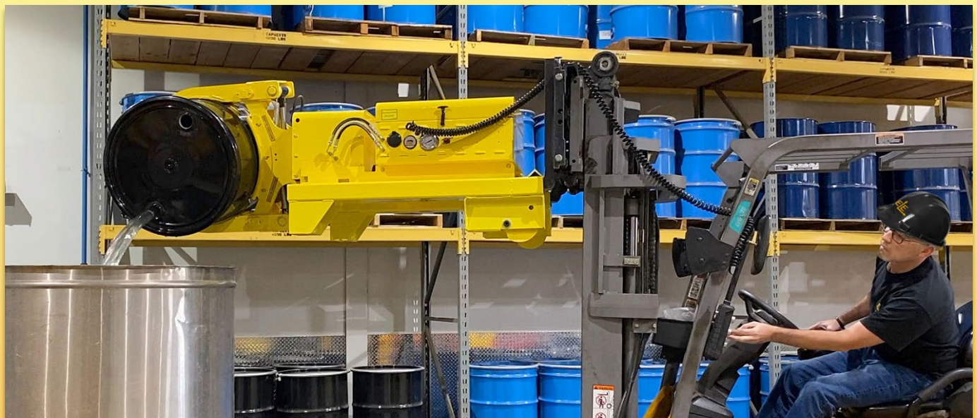
Using the EG2000RCR-QC Lift Truck Attachment to dump a steel drum into a tank
