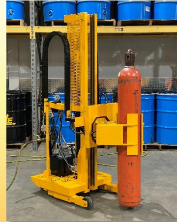
ELDR Air Powered Staddle Leg Model with CCR Clamp
