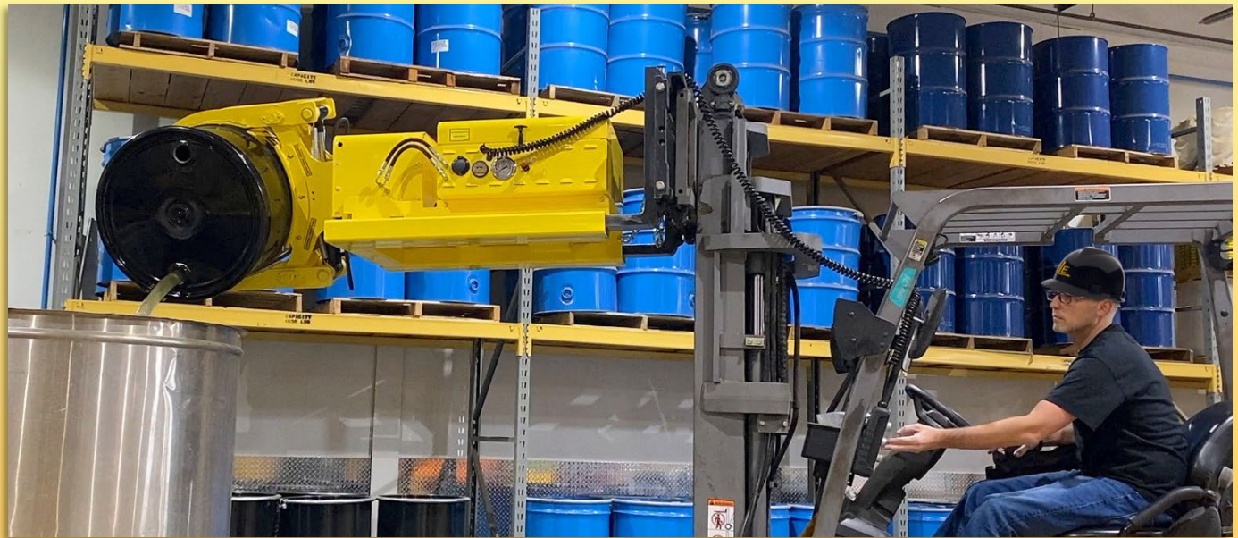
Using the EG2000RCR Lift Truck Attachment to dump a steel drum into a tank
