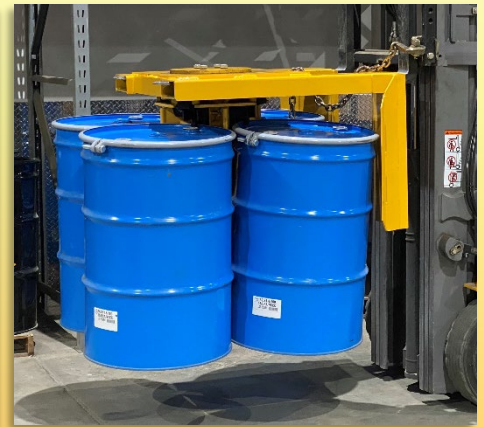
EL4F gripping and raising four full steel drums
