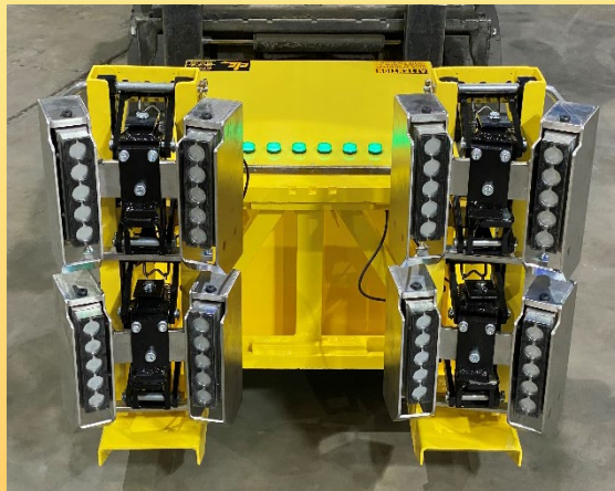
EG4M8DC2-F showing 8 magnets
