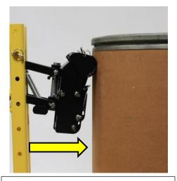
2. Push the unit forward so the fiber drum guards are contacting the paper portion of the drum.
