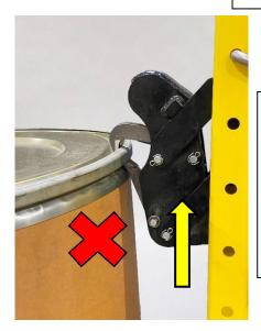
3. Maintain slight forward momentum while raising the drum so the lower clamping jaw maintains contact with the metal skirt. Do not allow the lower jaw to contact the paper portion of the fiber drum when elevating the drum.
