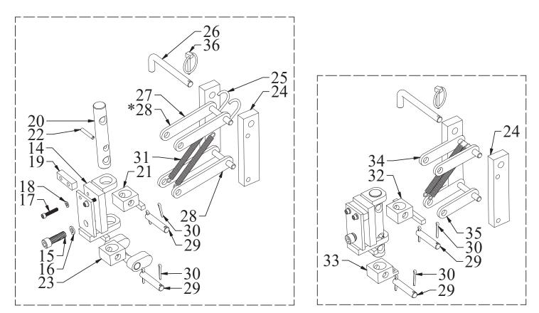
SEEN ON LEFT: **ERGO UNITS WITH A 5" BELT CRADLE** WILL PRIMARILY USE A 6" UPPER CLEVIS (#27) AND A 5-1/2" LOWER CLEVIS (#28). ALONG WITH A LOWER PIVOT BLOCK WITH OVAL STOP BARS (#23) AND AN UPPER PIVOT BLOCK WITH A 2-1/4" STOP BAR (#21).
