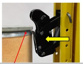
2. Then move the clamping mechanism forward so the lower jaw contacts the metal skirt under the drum's locking band and proceed to elevate the drum upward.
