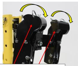
1. Ensure the fiber drum guards are in the forward position (closer to the clamp) and the cotter pins are locking the guards in place. The guards should always be in this position when handling fiber drums. The guards can be in the rearward position (closer to the mast) when handling steel or plastic drums.
