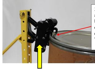
3. Elevate the clamping mechanism(s), allowing them to engage the locking band. After the clamp has fully engaged continue elevating the drum enough to ensure safe floor clearance. The drum can now be transported.
