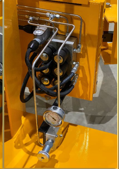
Side-rotation clamp w/ side shifter & adjustable clamping pressure
