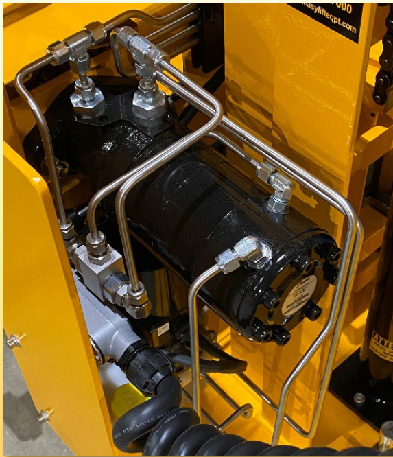
Side rotation anti-drift brake motor
