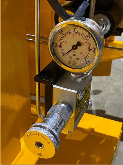
Side-rotation adjustable clamping pressure
