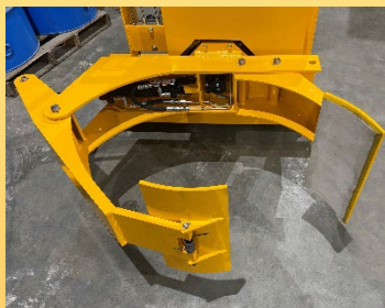
LRCR inner position clamping range 20" (51 cm) to 36" (91 cm) in diameter
