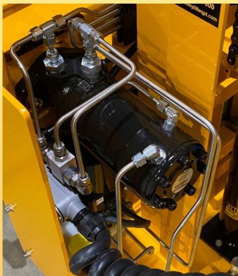
Side rotation anti-drift brake motor
