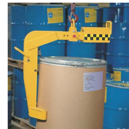
Model ETG1 can handle any chimed drum of all sizes. Adjustable counterweight keep drums of different weights and diameters perpendicular to floor when lifted. Used in conjunction with a hoist for palletizing drums off fill lines or placement in secondary containment pallets.
